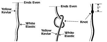
NOTE: THIS IS A VERY IMPORTANT STEP. IF YOU TIE A DIFFERENT TYPE OF KNOT THE SHOCK CORDS MAY SEPARATE DURING FLIGHT.
