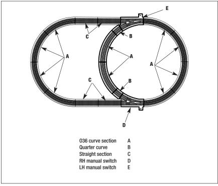
Figure 1. Inner Passing Loop track layout
