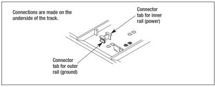
Figure 5. Connector tabs
