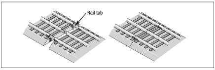
Figure 2. Joining the track sections
