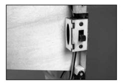
**8.** Install both ignition kill switches on the aircraft so that they are easily accessible from the outside of the plane.
