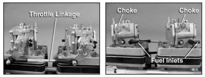
**5.** Control of the chokes will be necessary during start-up and operation. Make sure you have manual access or control of the chokes via a servo or mechanical linkage before completing installation of the DLE-222.
