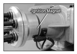
**3.** Next, set the engine at the beginning of the compression stroke. Note the position of the ignition magnet with engine inverted.
