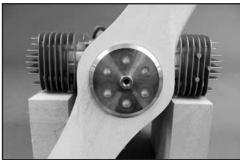
**4.** Place the propeller on the crankshaft at the one o'clock position.
