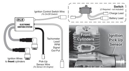
The Ignition Pick-Up Sensor Wire labeled in this picture of the engine corresponds to the *front* cylinders. Connect the Ignition Pick-Up Sensor Wire to the EIS that will control the ignition of the spark plugs installed in the *front* cylinders.
