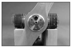
**6.** Remove the propeller from the engine and drill the outer hole on the drill press using a #35 (0.110"/ 2.81mm) drill bit as a pilot hole. Next use a 1/4" (6.28mm) drill bit to finish the hole. In order to achieve a clean finish on both sides of the propeller,
