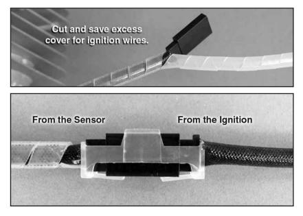
**2.** Install the silicone wire covers over the ignition pick up sensor leads coming from the engine (cut the excess silicon wire covers) and connect the leads to the pick up sensor leads from the Electronic Ignition Modules. Secure the connections with the included three pin connector securing clips.
