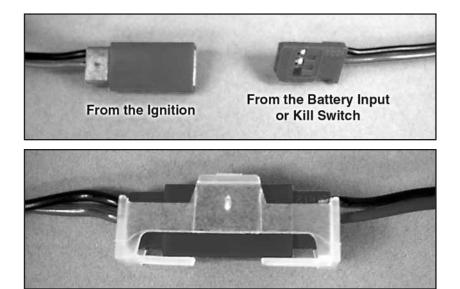
**3.** Connect the ignition kill switch leads to the red connector from the ignition control module using the lead from the kill switch or with the included three pin connector with pig tail. Use the included three pin securing clips to secure the connections.
