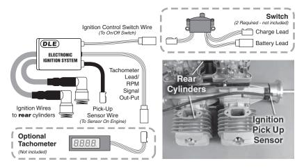
The Ignition Pick-Up Sensor Wire labeled in this picture of the engine corresponds to the *rear* cylinders. Connect the Ignition Pick-Up Sensor Wire to the EIS that will control the ignition of the spark plugs installed in the *rear* cylinders.
