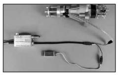
Many of the DLE Ignition modules have an additional lead to plug into the optional tachometer. If your ignition module does not have this additional lead, the digital tachometer can still be used. Simply use the Y-harness (included with the Digital
