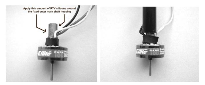
**NOTE:** Photo shows installation using a carbon fiber tube, with 7mm OD, 5mm ID (EFLM1963 available separately). This is an option for mounting the motor. You can cut down the carbon fiber tube to meet your specific needs and attach to your foam or wood airplane with glue.
