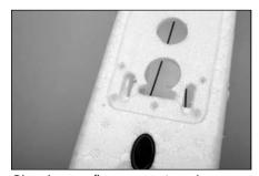
Glue the rear float mount into the fuselage using epoxy, making sure not to get epoxy in the screw holes. Go to the assembly and installation section when done mounting the rear float mount into your Super Cub.
