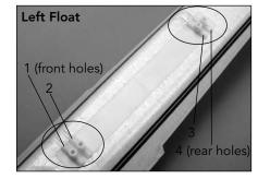
• Install the landing gear with the wider top portion into the front holes on the floats. Next install the front spreader wire into the second holes on the floats. Install the rear spreader wire into the third holes on the floats. Finally, install the rear landing gear legs with the narrower top portion into the rear holes on the floats.
