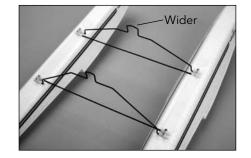
• Install the eight 3mm x 10mm Phillips head machine screws into the floats making sure the screws are tightening against the flat spots on the wires.
