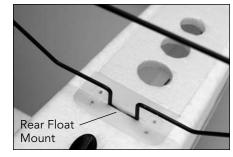
• The Super Cub LP (blue Super Cub with Li-polymer battery) comes with the rear float mount pre-installed in the fuselage. If you are attaching your Super Cub floats to an original red Super Cub (HBZ7100), a rear float mount will have to be installed into the fuselage. This is a separate part that has been included with this float set. Please see page 9 for installation instructions.
