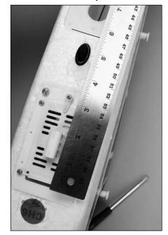
Press hard enough to leave marks in the foam on the fuselage to indicate what foam needs to be removed. Set the rear mount aside, then slowly cut away where the foam is compressed by the rear float mount until the mount is flush with the bottom of the fuselage.
