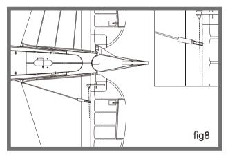
4. Turn over the fuselage so the bottom faces up and feed the connector wires thorough the hole in the fuselage. Secure the wing in place using 4 wing screws.
