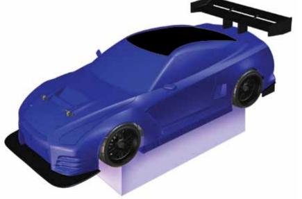
Perform a control test with the vehicle. wheels off the ground. If the wheels rotate after the vehicle is powered ON, adjust the "TH, Trim" knob until they stop. To make the wheels move forward, pull the trigger. To reverse them, wait for the wheels to stop. then push the trigger. When moving forward, the wheels should maintain a straight line without any steering wheel input. If not, adjust the "ST. Trim" knob so the wheels maintain a straight line without having to turn the steering wheel.
