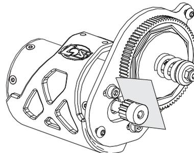
1. Loosen the motor screws and slide the motor back.
