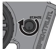
Turn the ST RATE knob counter-clockwise to reduce the sensitivity.
