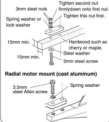
Make sure that these mounting beams are accurately aligned and firmly integrated with the airframe, reinforcing the adjacent structure to absorb vibration. Use 4mm or larger steel screws, preferably Allen type hexagon socket head cap screws, with washers and locknuts, for bolting the engine to the bearers.
