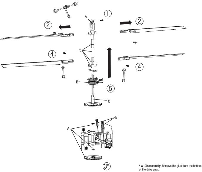
**Re-assembly:** Add a drop of white glue to the bottom of the drive gear and inner shaft.
